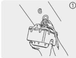
Attach hoist with a rated lifting shackle and secondary support tether or optional installation bracket to ceiling structure.
