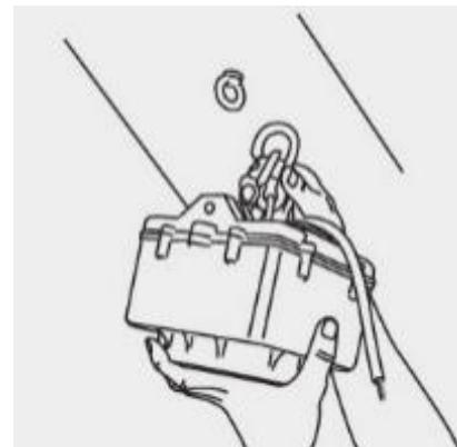
Hoist can be hung directly from the attachment eye on the top of the hoist body. A secondary safety tether is required if this fixing method is used.
