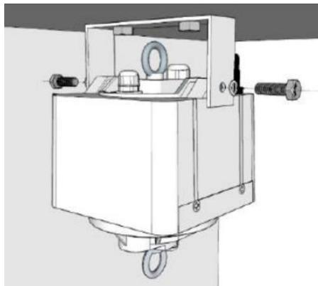
Hoist can be rigidly secured to building structure via a bolted, u-shaped ceiling bracket.
