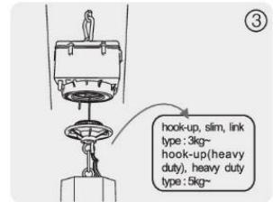
Attach light fitting to the connection point on the underside of the hoist.
