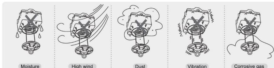
Avoid installing where there is high moisture, high wind, excessive dust, vibration and/or corrosive gas.
