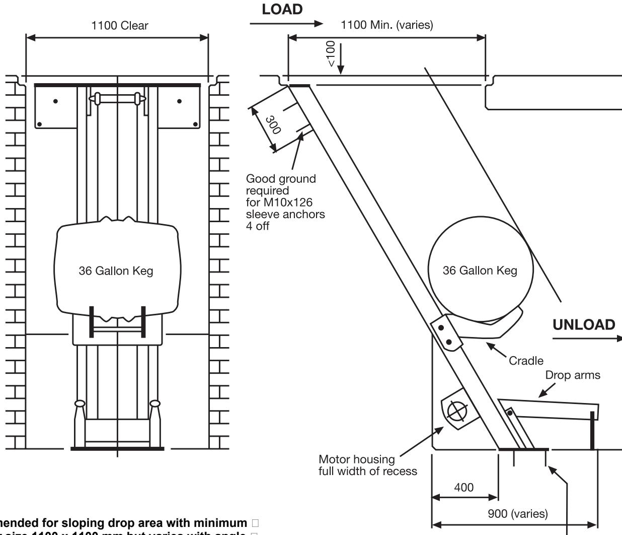
Recommended for sloping drop area with minimum trapdoor size 1100 x 1100 mm but varies with angle.
