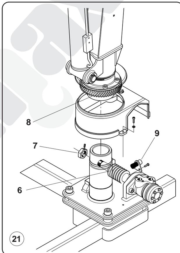
*It is important to check that the worm gear reducer has a correct axial backlash. This can be made, with the crane at standstill, the boom in horizontal position. Pushing the boom aside on the left and on the right by hand, you can notice if the axial backlash between the wormshaft (6) and the wormgear (8) is too great. In this case it has to be reduced, tighten the nut (7) accordingly. Grease the gear with the suggested product and replace the grease spreader (9), if worn out.*
