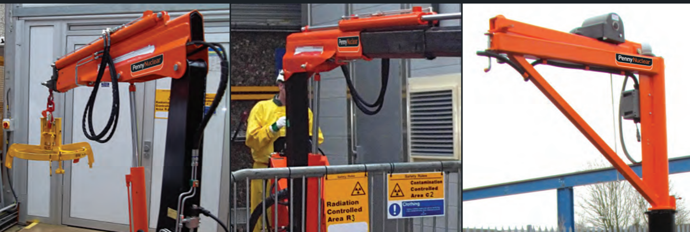
Bradwell hydraulic export crane
