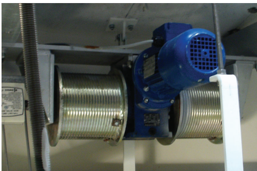
LEFT: example of a motorised winch installation
