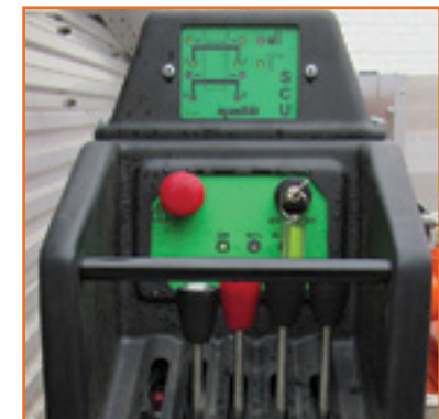
SCU: Stability Control Unit with LME04
