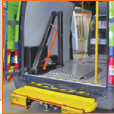
Rear door box section frame with alloy top
