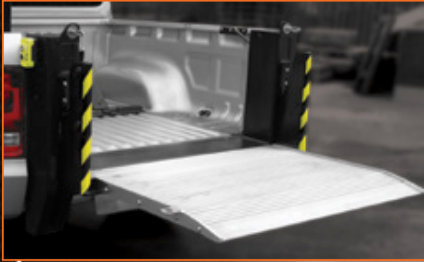
Lightweight aluminium platform
