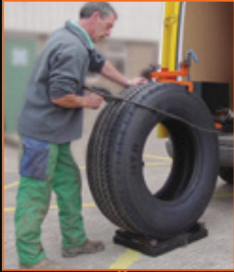
Optional top clamp for tyre re-grooving
