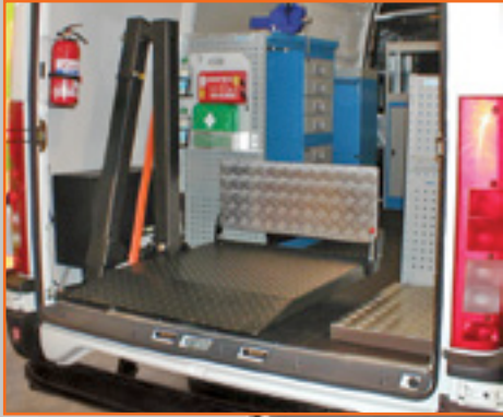
Bespoke lift with safety stop
