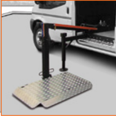
Sidedoor box section frame with alloy top
