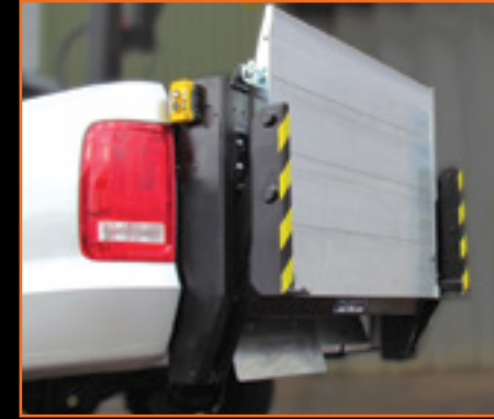
EL 4 x 4 stowed position; excellent ground clearance
